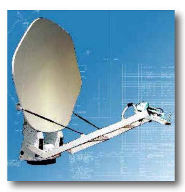
The CPI Satcom & Antenna Technologies Inc. (CPI SAT) lightweight 2.4-meter mobile antenna is designed for worldwide transmit and receive operation in C, X, Ku and Ka-band. This mobile antenna consists of a carbon fiber composite reflector and back beam mounted on a cable-driven, elevation-over-azimuth positioning system. This results in an antenna with superior stiffness and high performance under wind loading conditions.
